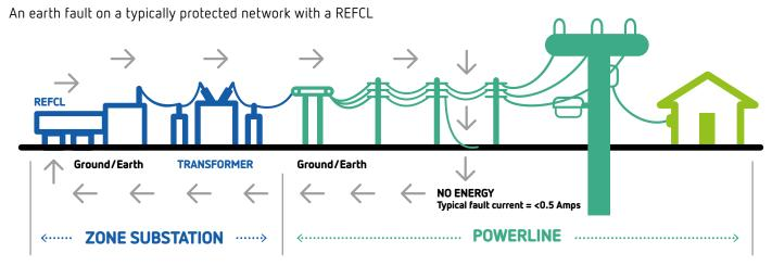
When an earth fault occurs a REFCL detects and cuts the energy flow within a tenth of a second on the powerline that has the fault. This reduces the possibility of a fire being started.
