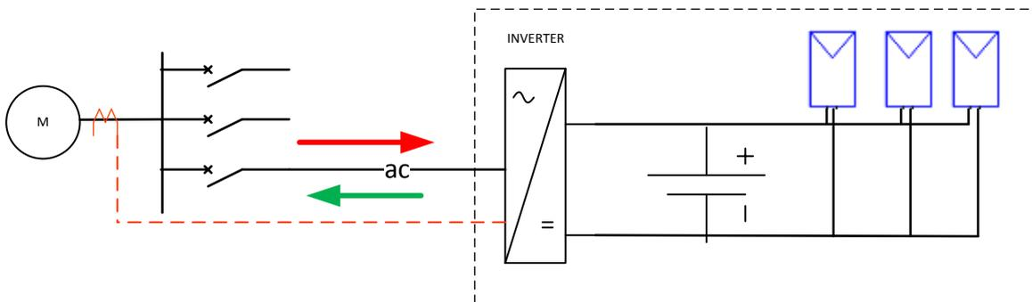
Installed Capacity = the common inverter rating
