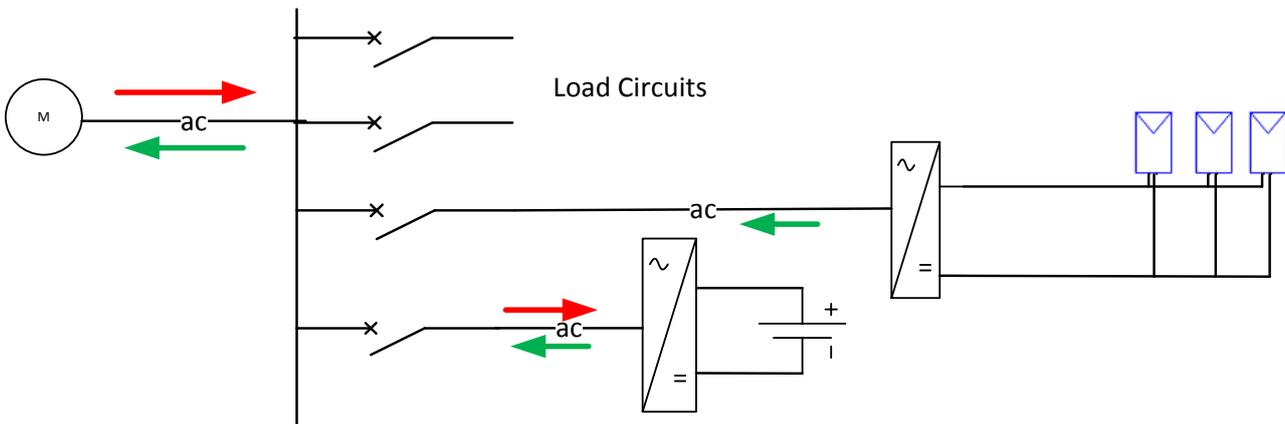
Installed Capacity = solar inverter rating + battery inverter rating
