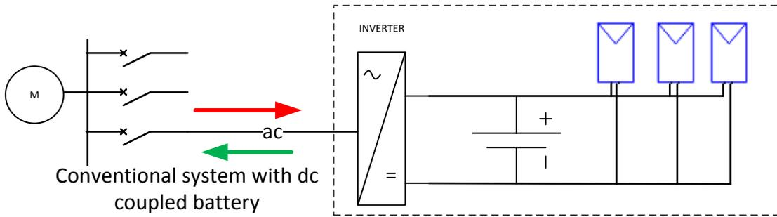
Figure 2 Example of a DC coupled solar and battery storage system
