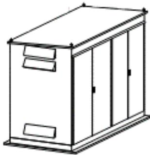
Figure 14. Ring Main Unit - Isometric view
