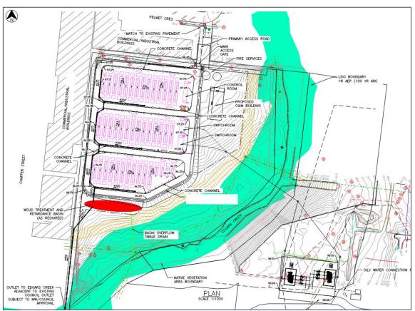
Figure 1: Proposed BESS layout (extract from drawing TTS-CIV-001)
